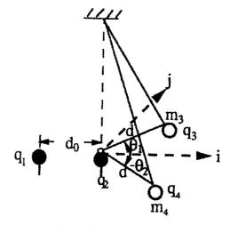
Fig. 2 Fixed charge electroscope.
