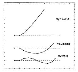
Fig. 7 Lowest 3 natural modes and frequencies of the electrostatic string.
